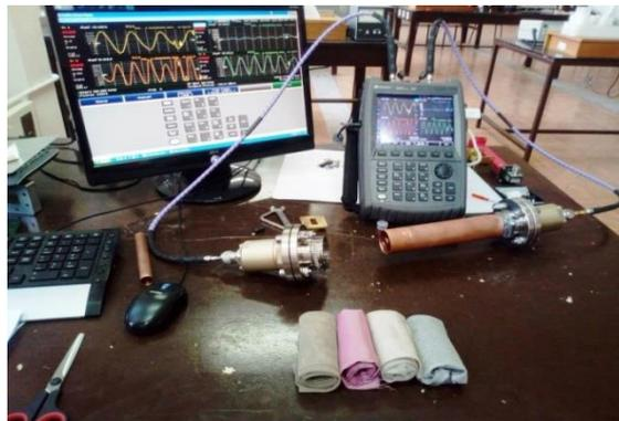
**Figure 1.** A photo of the microwave measurement setup.
