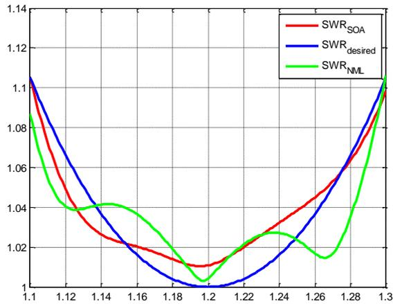
**Figure 5.** Standing wave ratio for the desired, NML and for the SOA obtained design vs. frequency for fixed  $Z_0$ .
