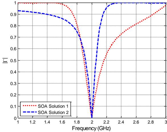
**Figure 4.** The reflection coefficient magnitude for solutions obtained by SOA vs. frequency for the double stubs matching
