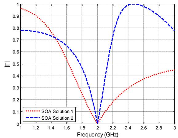
**Figure 3.** The reflection coefficient magnitudes obtained by SOA versus frequency for a single short circuit shunt stub.
