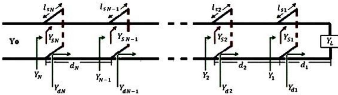
Figure 1. General N parallel stubs connection [9].
