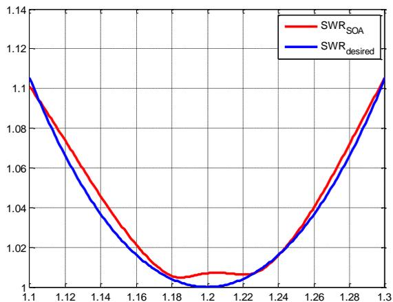
**Figure 6.** Standing wave ratio for the desired and for the SOA obtained design vs. frequency for variable  $Z_0$ .
