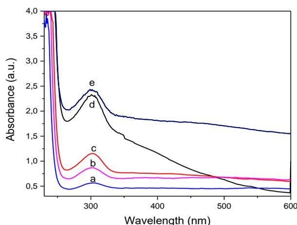
Figure 3. UV–Visible spectra of AgNP coating solutions at different AgNO<sub>3</sub>/CMS concentrations (a.F025, b.F05, c. F1, d. F2, e.F5)
