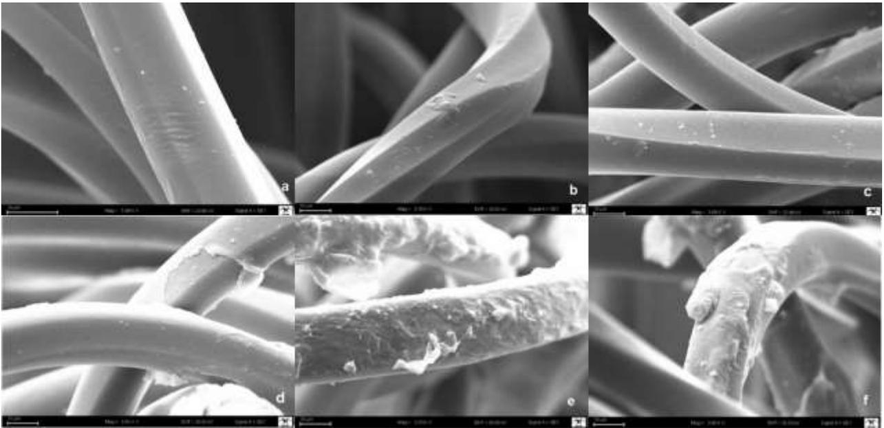
**Figure 4.** SEM images of AgNPs coated composite PA yarns (a. Uncoated yarn b. F025, c. F05, d. F1, e. F2, f. F5, Scale: 10  $\mu\text{m}$ )
