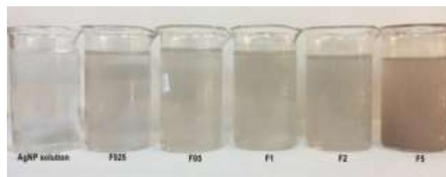
Figure 2. Silver nanoparticle coating solutions at different AgNO<sub>3</sub>/CMS concentrations.
