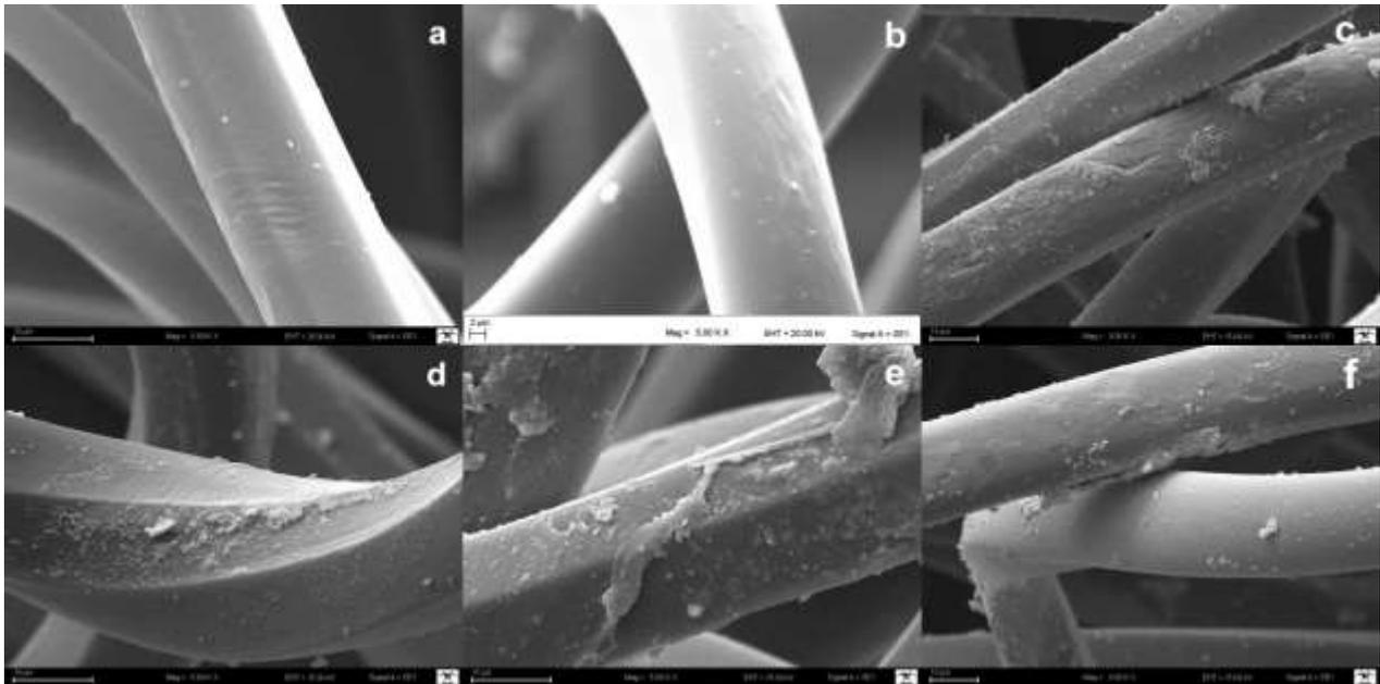
**Figure 5.** SEM images of AgNPs coated PA composite yarns (a.Uncoated yarn b. 1h, c. 2h, d. 3h, e. 4h f. 5h, Scale: 10  $\mu\text{m}$ )
