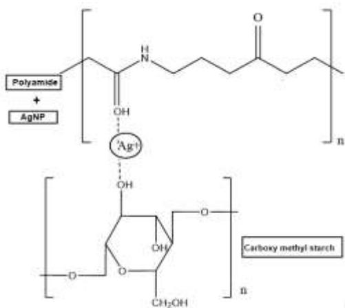
Figure 7. Schematic formation of AgNPs coated PA yarns
