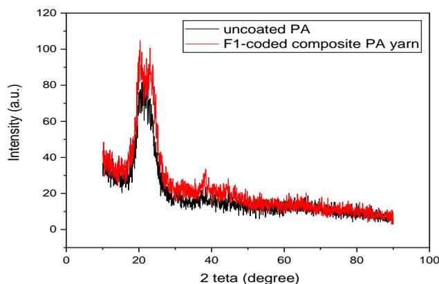
Figure 8. XRD patterns of uncoated and F1-coded composite PA yarn
