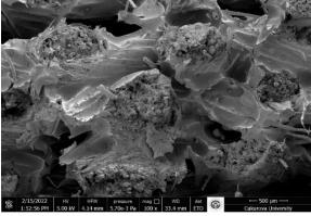
Figure 15. JE composites at 90°C post cure temperature SEM micrograph
