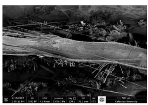
Figure 17. JBE composites at 90°C post cure temperature SEM micrograph
