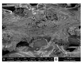
Figure 9. JE composites at 50°C post cure temperature SEM micrograph
