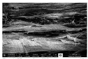
Figure 16. BE composites at 90°C post cure temperature SEM micrograph
