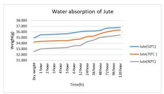
Figure 6. Water absorption analysis results of Jute composite
