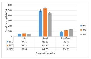
Figure 4. Tensile test results
