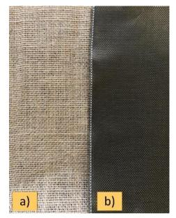
Figure 1. Fabric specimens: a) Jute fabric b) Basalt fabric
