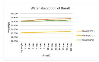
Figure 7. Water absorption analysis results of Basalt composite
