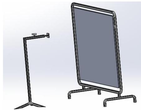
Figure 7. Sensing range adjustment board for ultrasonic sensor
