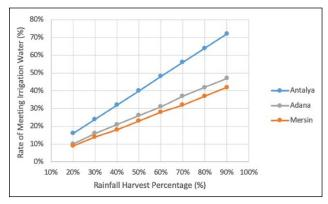
**Figure 2**. Rates of meeting irrigation water requirement in different provinces according to TS 825 based on rainfall harvest rates.
