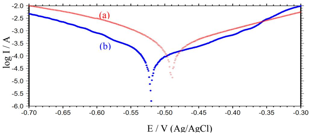
**Figure 7.** The potentiodynamic polarization curves of MS electrode in 0.5 M HCl (a) and 5mM 2I4MTA5C containing 0.5 M HCl (b) solutions after 168 h.
