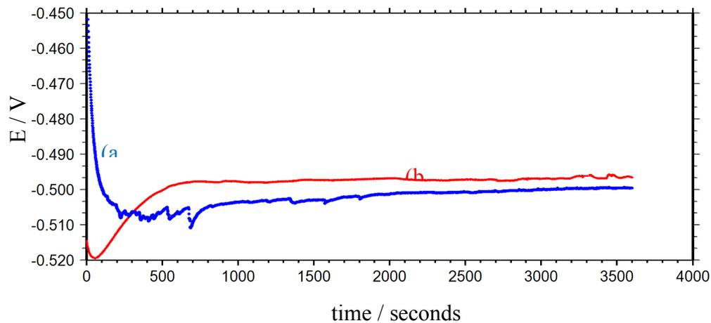
**Figure 2.** The open circuit potential of MS in 0.5 M HCl (a) and containing 5mM 2I4MTA5C (b) solutions.
