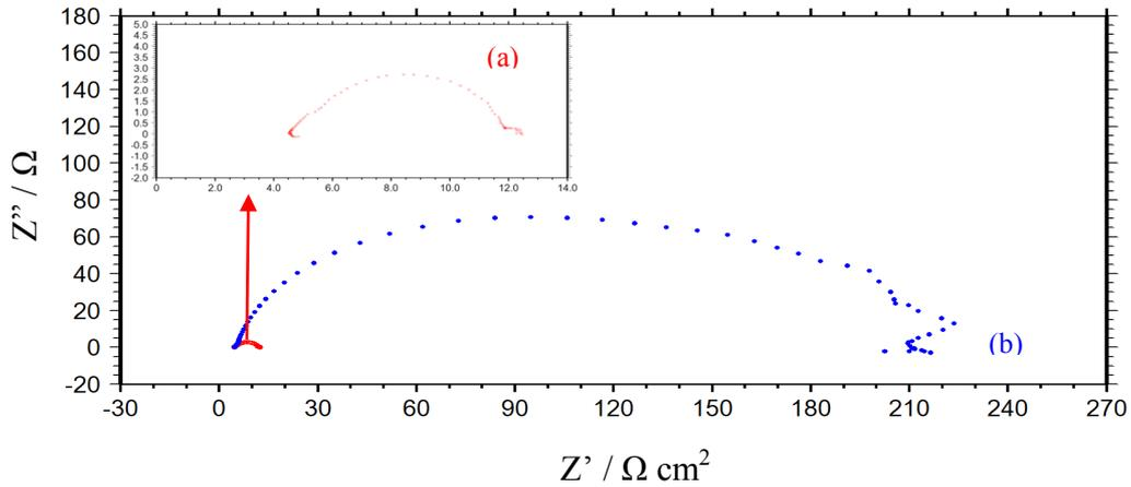
**Figure 4.** The Nyquist plots of MS electrode in 0.5 M HCl (a) and 5mM 2I4MTA5C containing 0.5 M HCl (b) solutions for 168 hours immersion period.
