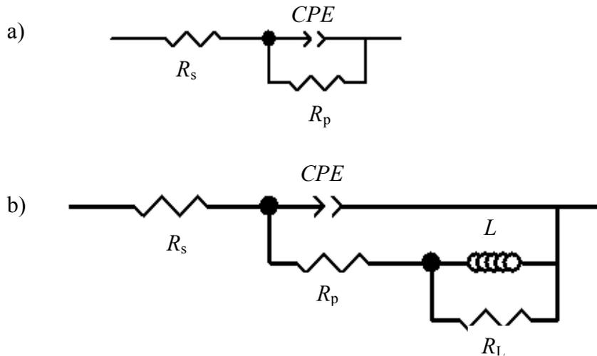
**Figure 5.** Electrical equivalent circuit diagrams used to modeling MS/HCl (a) and MS/HCl+2I4MTA5C (b) solutions interfaces. The solution resistance is  $R_s$ ; the polarization resistance is  $R_p$ , the constant phase element is CPE, the inductance is  $L$  and  $R_L$  is the resistance due to the adsorbed species.
