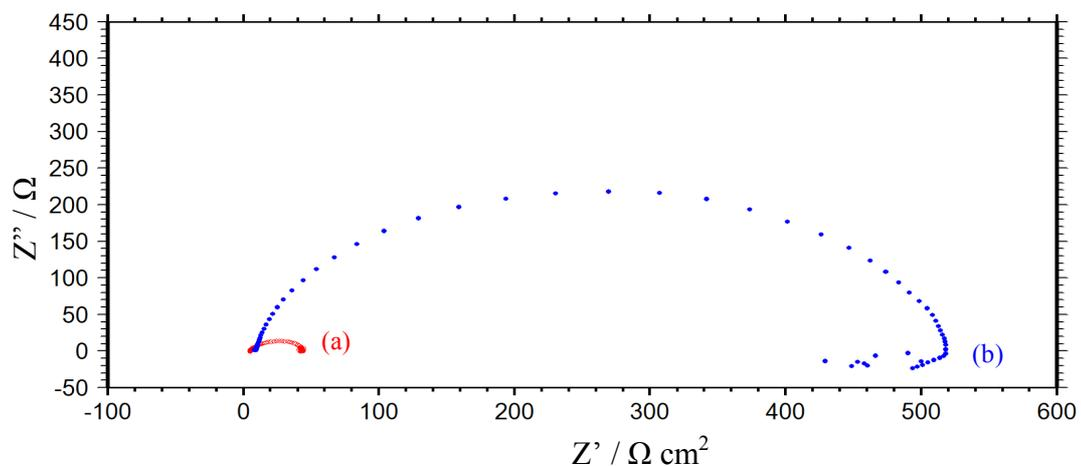
**Figure 3.** The Nyquist plots of MS electrode in 0.5 M HCl (a) and 5mM 2I4MTA5C containing 0.5 M HCl (b) solutions for 1 hour immersion period.
