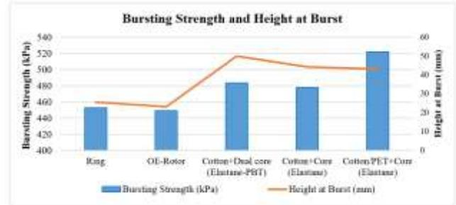
**Figure 10.** Bursting strength and height at burst of denim fabrics**Table 12.** SNK results for bursting strength values of denim fabrics
