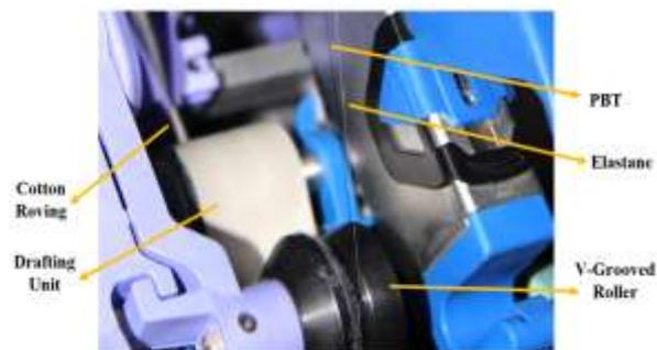
Figure 1. Cotton / PBT-elastane dual core ring yarn production
