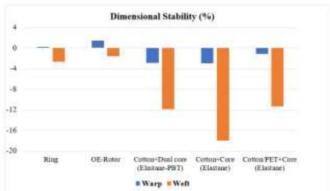
Figure 6. Dimensional stability of denim fabrics in warp and weft direction (%)
