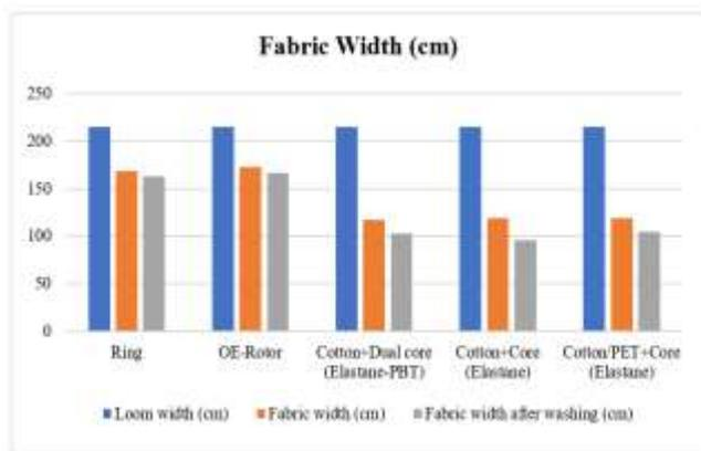
Figure 7. Denim fabric widths before and after washing
