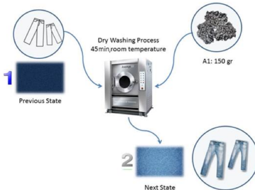
Figure 2. Dry Washing Process
