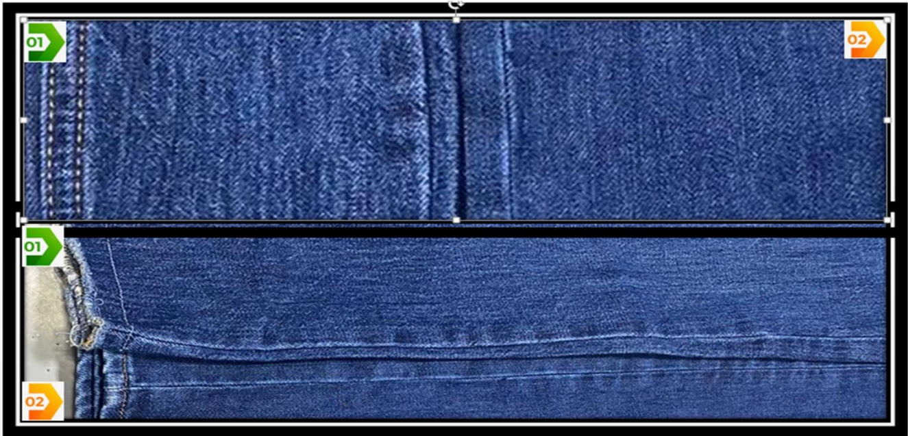
Figure 6. Aging Effect Study With Different Materials, 1) Pumice Stone and KMnO_4 , 2) Al_2O_3 Based Abrasive Slurry
