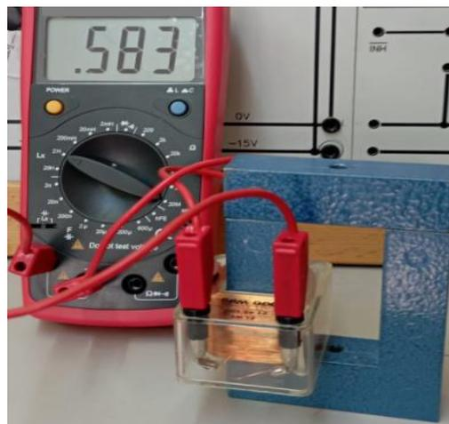
**Figure 10.** Measuring the inductance of the silicon steel core coil with an LCR-meter
