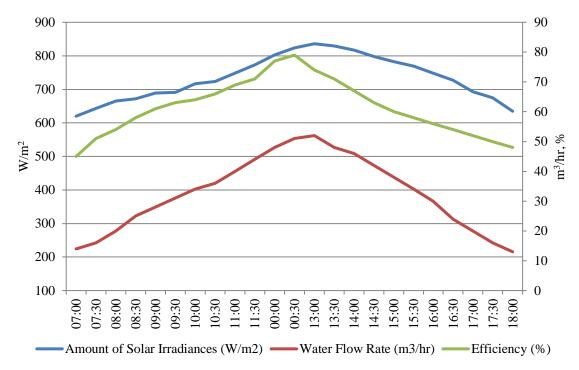
Figure 4: Performance of Tracking Solar Pumping System for Cloudy Day
