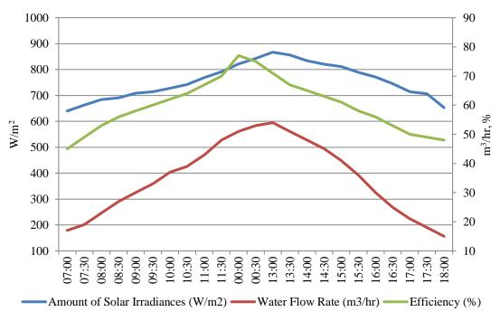
Figure 3: Performance of Fixed Solar Pumping System for Sunny Day
