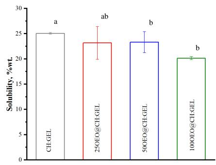
**Figure 5.** The solubility of films against water for 48 h. Different letters in the bar indicate a significant difference (p < 0.05).
