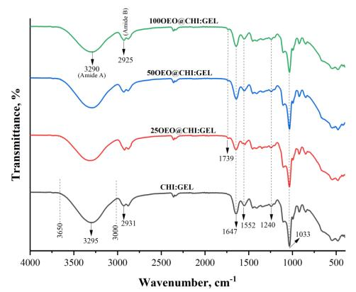
Figure 4. FTIR spectrums of CH:GEL and different concentrations of OEO incorporated into OEO@CH:GEL films.
