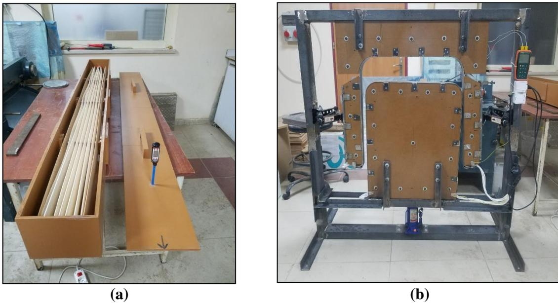
Figure 3. Steam cabin (a) and bending press (b)
