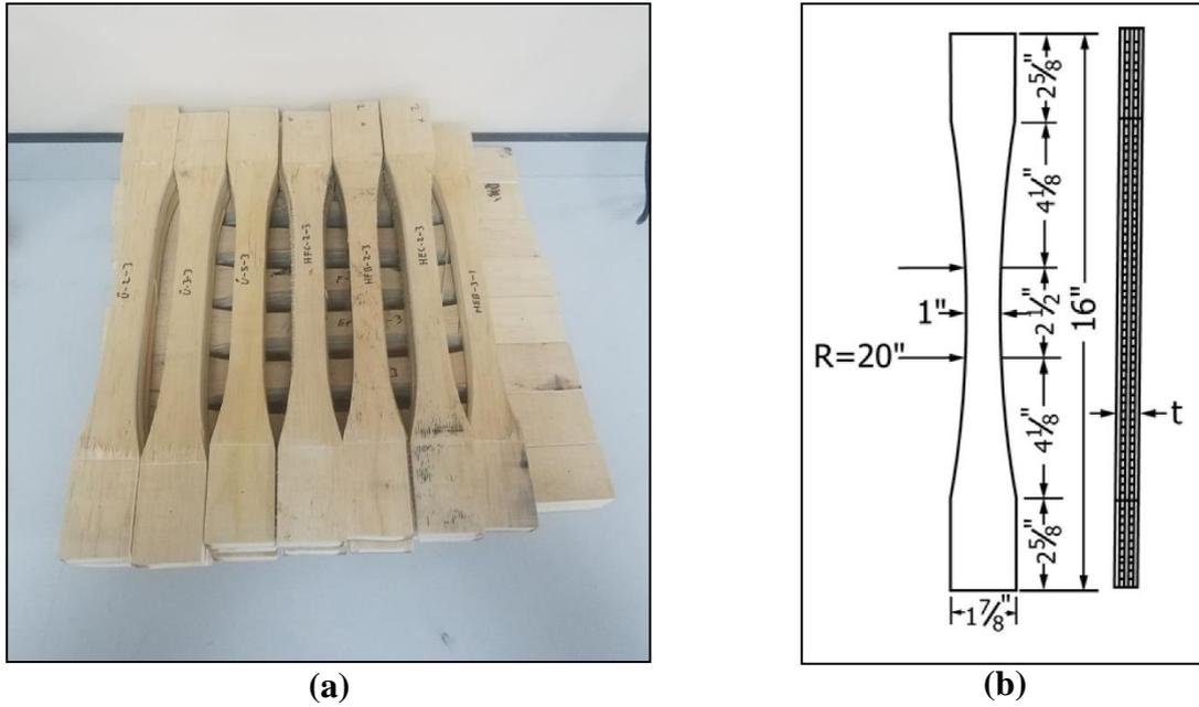
**Figure 6.** The test sample (a) and technical drawing (b)
