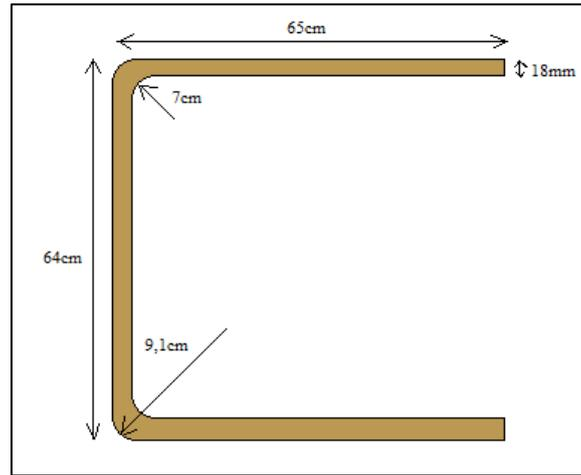
**Figure 4.** Bending test sample
