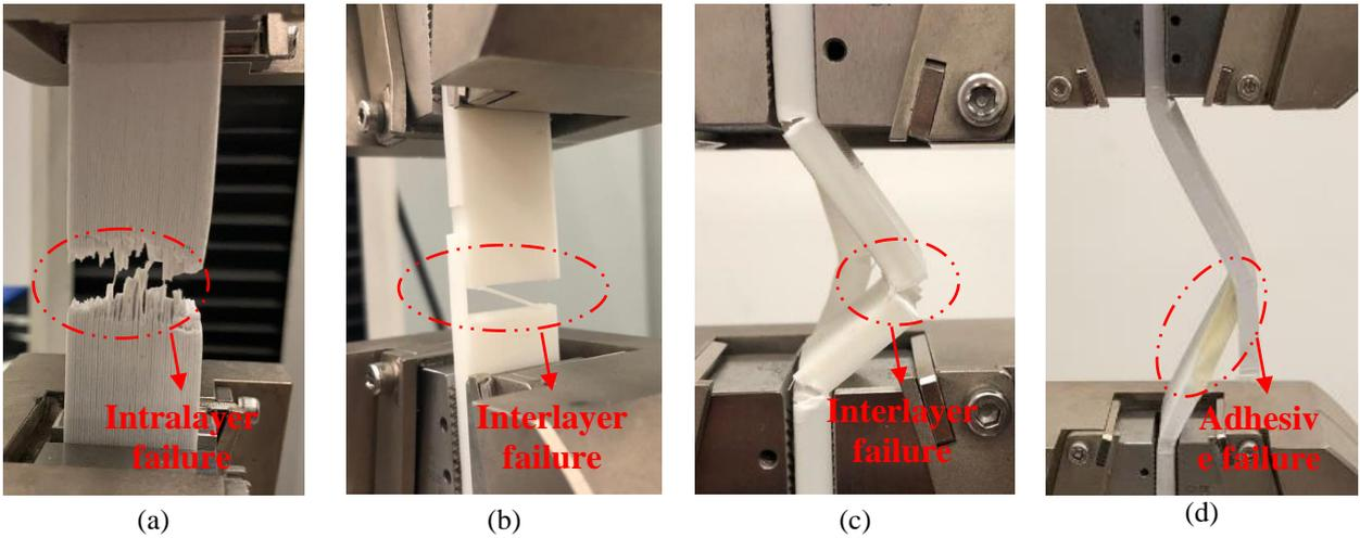
Fig. 3. Illustration of different experiments (a) tensile test of a single PLA specimen – O0T, (b) tensile test of a single PLA specimen - O90T, (c) compression test of a single PLA specimen – O90C, and (d) compression test of the scarf joint specimen - O45A30.
