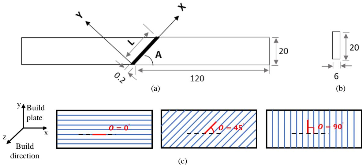
Fig. 1. Scarf joint specimen configurations (a) Top view of general configuration (b) Cross-sectional dimensions, (c) Three raster orientations of  $0^\circ$ ,  $45^\circ$ , and  $90^\circ$  in 3D printing (from left to right, respectively). The build plate is on the  $xy$ -plane and the specimens are printed in  $z$ -direction.
