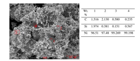
Figure. 8. EDS analysis of electroless Ni coated SiC powders.
