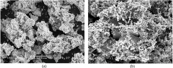
Figure 7. SEM images of electroless Ni coated SiC powders at different magnifications.
