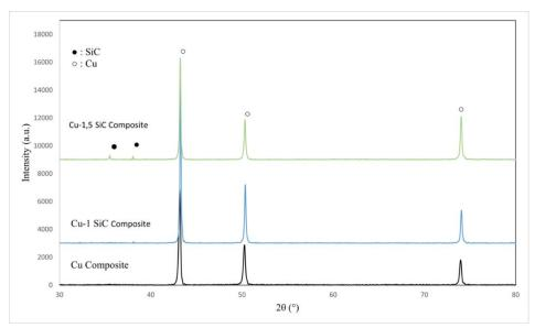
Figure 11. XRD patterns of cemented Cu and Cu 1-1.5 wt.% NiSiC composites
