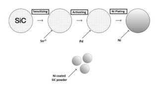
Figure 2. Schematic representation of Electroless Ni coating on SiC.
