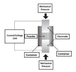
Figure 3. Schematic representation of sintering by ECAS Method [11], [15].
