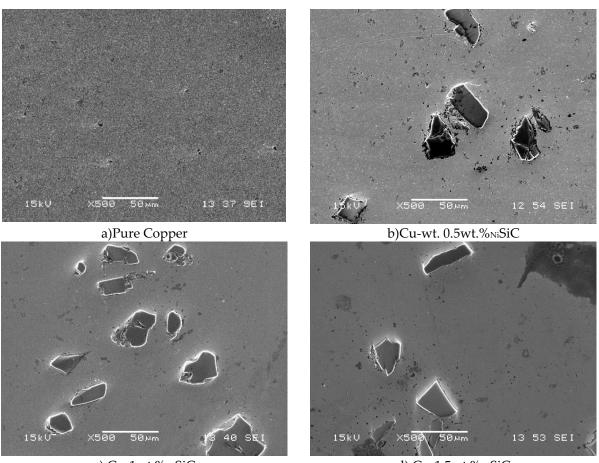
c) Cu-1wt.%<sub>Ni</sub>SiC d) Cu-1.5wt.%<sub>Ni</sub>SiC **Figure. 9.** SEM images of cemented Cu and Cu- 0.5-1-1.5 wt.% Ni SiC composites
