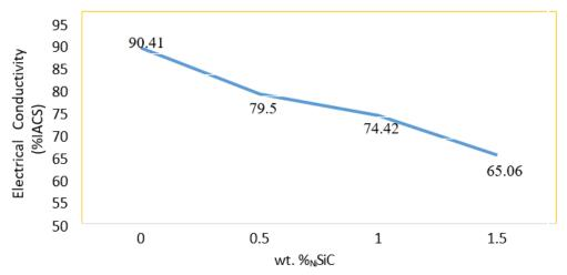
Figure 12. Electrical conductivity (%IACS) variation of cemented Cu and Cu-Ni SiCcomposites
