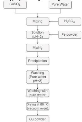
Figure 1. Schematic representation of the production of cemented copper powder
