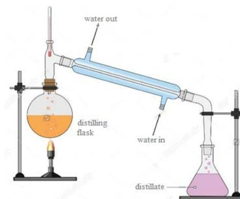
Figure 9. Simple distillation setup (Gavahian and Farahnaky, 2018)
