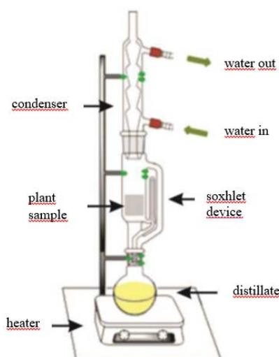
Figure 12. Soxhlet assembly (Guntero et al., 2017)
