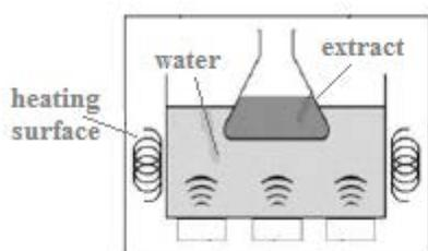
Figure 15. Ultrasonic assisted extraction system (Samaram et al., 2013)
