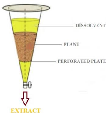
Figure 5. Percolation apparatus (Alara et al., 2021)
