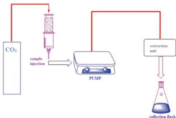
Figure 14. Supercritical fluid extraction system (Hussain et al., 2019)
