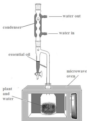
Figure 16. Microwave assisted extraction (Elguea-Culebras et al., 2022)
