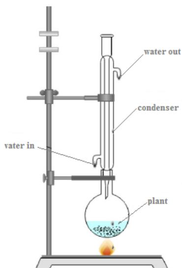
Figure 7. Reflux extraction techniques (Abd Aziz et al., 2021)
