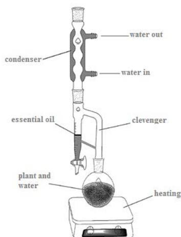
Figure 10. Water distillation device Clevenger (Elguea-Culebras et al., 2022)
