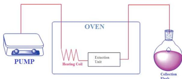
Figure 13. Pressurized liquid extraction system (Alara et al., 2021)
