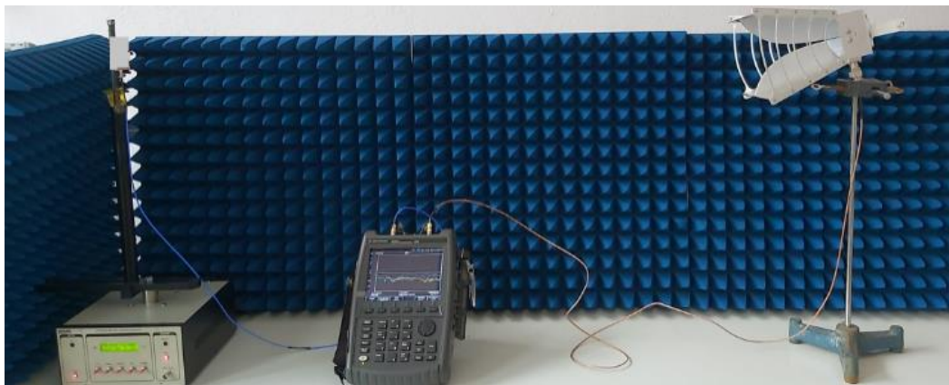
Figure 6. The Semi-Anechoic Chamber Measurement Environment
