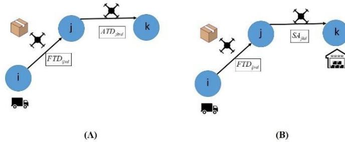
**Figure 10.** Movements of the drone after servicing a customer: A) land on any truck at another customer, B) return to the warehouse
