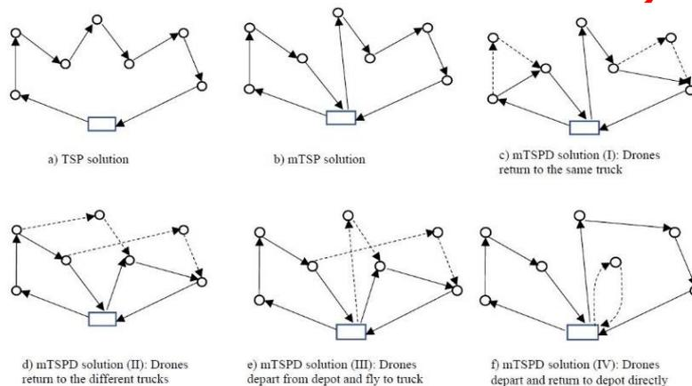
Figure 7. TSP, multi-TSP, and multi-TSP-DRONE feasible solutions are shown (Kitjacharoenchai et al. [33])
