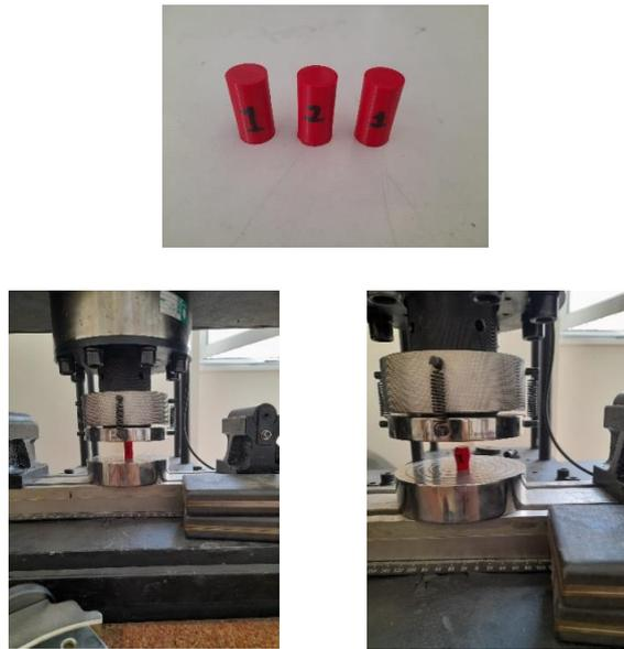
**Figure 1.** Compression Specimens Used in the Experiments
