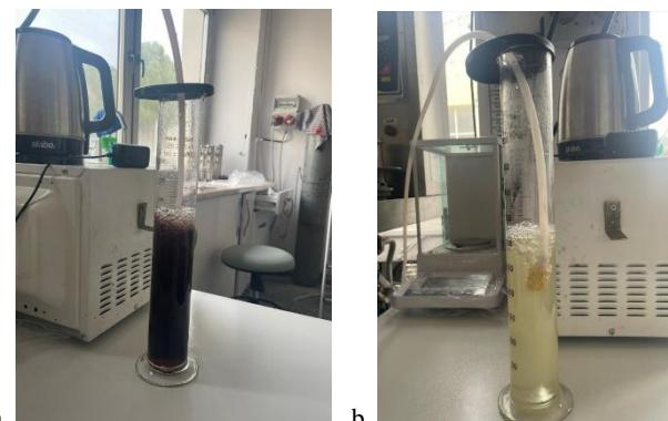
**Figure 6.** Ozonation of sample wastewater: a. Colored wastewater
