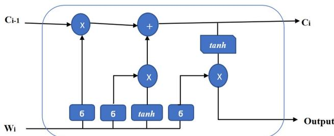
Fig. 5: LSTM model
