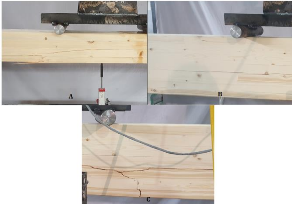
Figure 7. Typical Failure Modes of Specimens (A) Shear Failure of Splitting of Timber (B) Splitting of Timber (C) Shear Failure of Splitting of Timber
