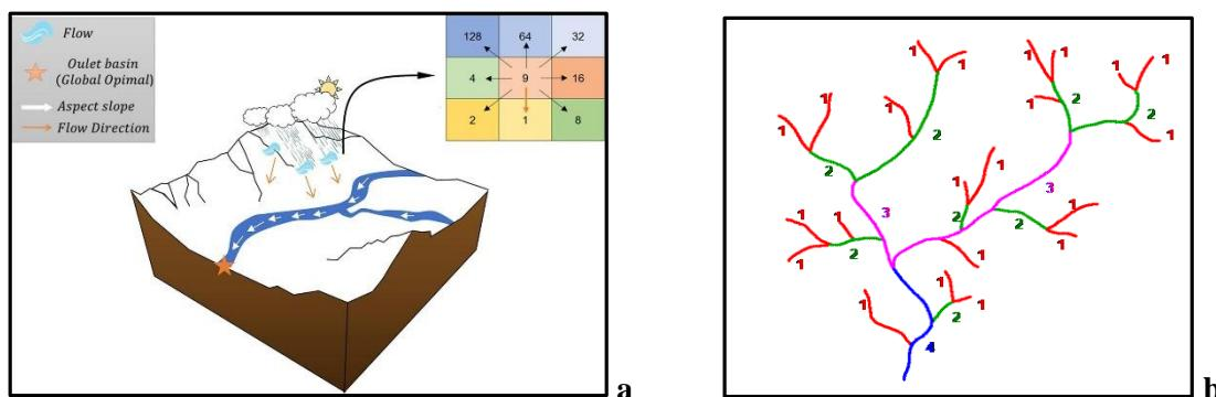
Figure 3. a) Flow to outlet of basin to schematic shame (Karami et al., 2021), b) Diagram of the stream order and values procedure used by DEM (Strahler, 1957)
