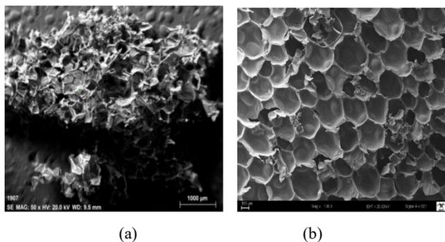
**Figure 1.** SEM images of biomass-based PU foams (a) and petroleum-based PU foams (b).
