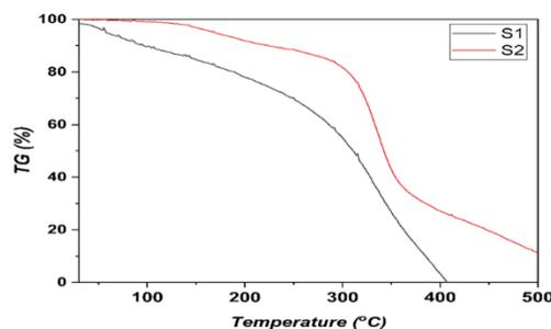
**Figure 2.** TGA thermograms of biomass-based PU foam (S1) and synthetic PU foam (S2).
