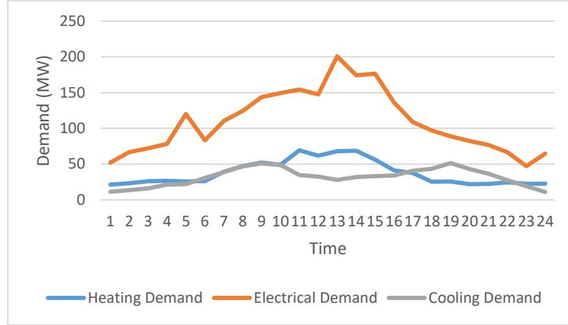
**Figure 2.** The electrical, heating and cooling demand
