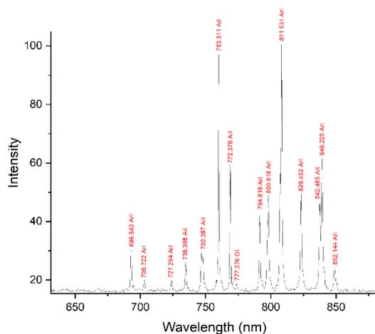
**Figure 2.** Optical emission spectrum of argon plasma.
