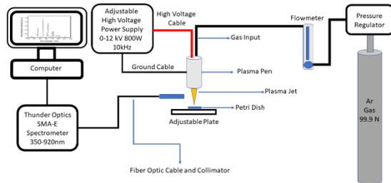
**Figure 1.** Atmospheric cold pressure plasma jet setup.
