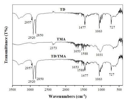
Figure 3. The FTIR spectra of the TD, TD/TMA and TMA
