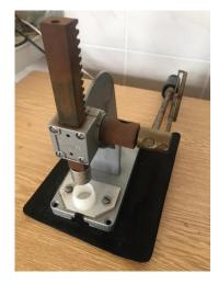
**Figure 1.** Pressing of TD/TMA after impregnation.
