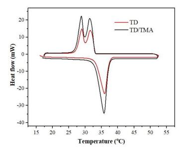
Figure 4. DSC thermograms of TD and TD/TMA
