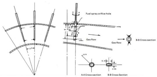
Fig. 9. Spray bar position configuration.
