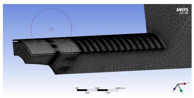
Fig. 16 Afterburner mesh model and mesh statistics.
