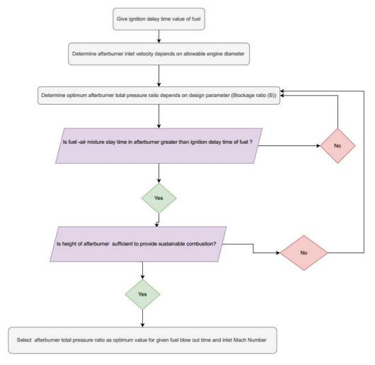
Fig. 2. Afterburner optimization algorithm.
