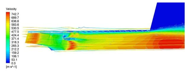
Fig. 17 Mid-plane velocity distribution of afterburner.
