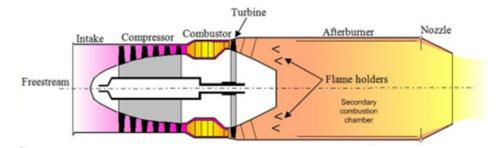
Fig. 3. Afterburner jet engine schematic view.
