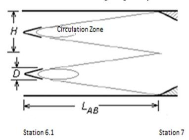
Fig. 11. Typical vee-gutter configuration.
