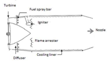
Fig. 5. Main features of a typical afterburner.
