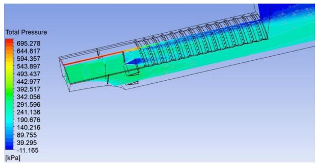
Fig. 18 Total pressure contours.
