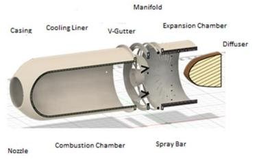
Fig. 13. Afterburner components.
