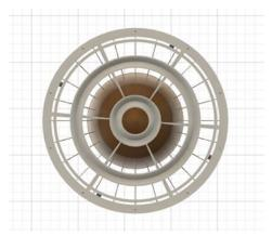
Fig. 12a. Vee-gutter 3D front view.
