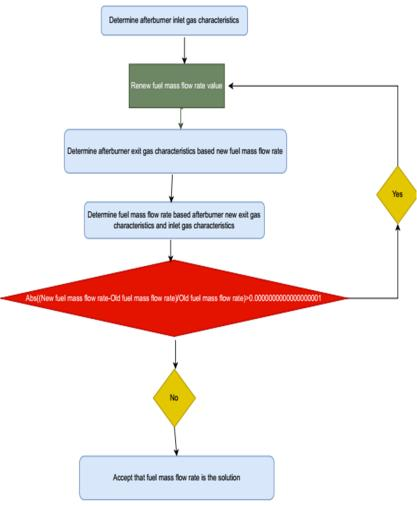
Fig. 4. Algorithm used to calculate fuel mass flow rate.
