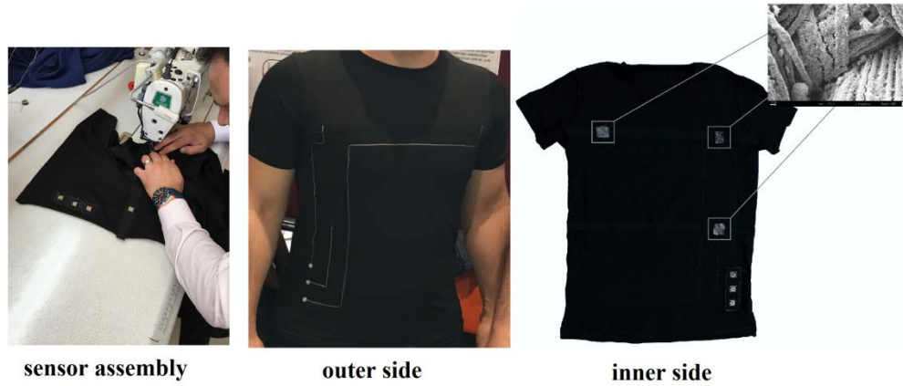
Figure 6. Design and Assembly of PET-PEDOT Based ECG Sensor on Garment
