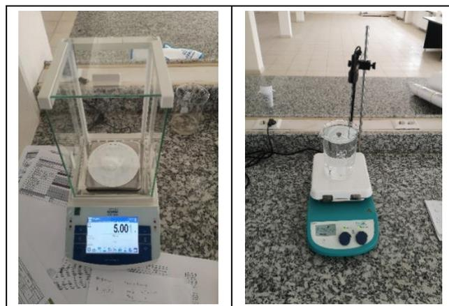
Figure 1. Preparation of solutions; weighing on precision balance and mixing on magnetic stirrer with heater.
