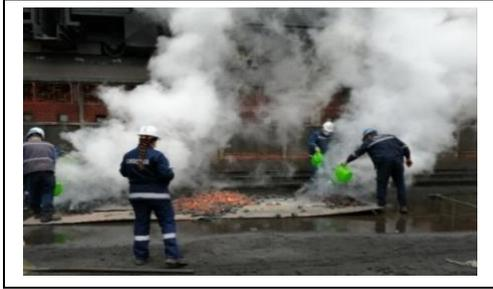
Figure 3. The moment of application of boron solution to the hot coke.
