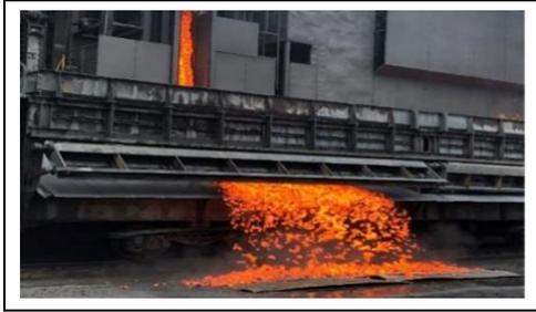
Figure 2. The hot coke was taken on sheet metal.
