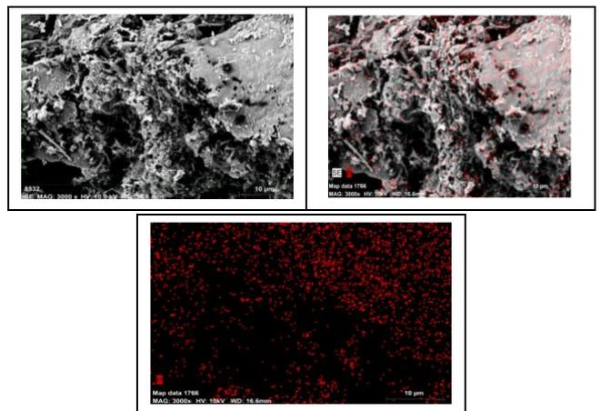
Figure 9. Mapping analysis of the coke sample quenched with Disodium Octaborate Tetrahydrate solution at a concentration of 7 g/l.
