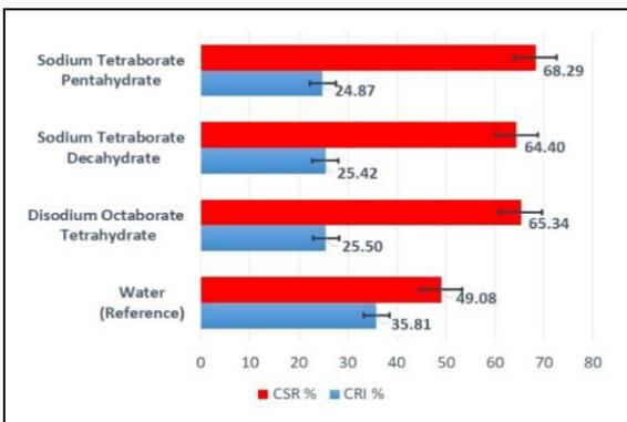
Figure 7. % CSR and % CRI values of solutions prepared using different boron products with a concentration of 10 g/l and water-quenched coke samples.
