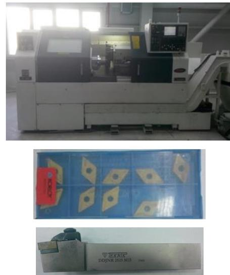
Figure 1. The cutting tool, tool holder and CNC lathe
