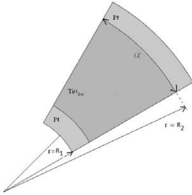
Figure 2. The unsaturated cylindrical-cut memristor topology
