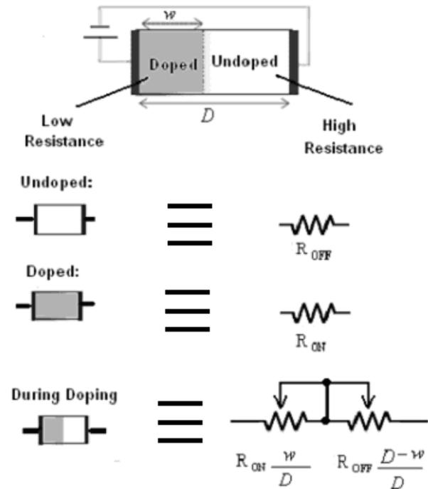
**Figure 1.** TiO<sub>2</sub> memristor and its equivalent circuit
