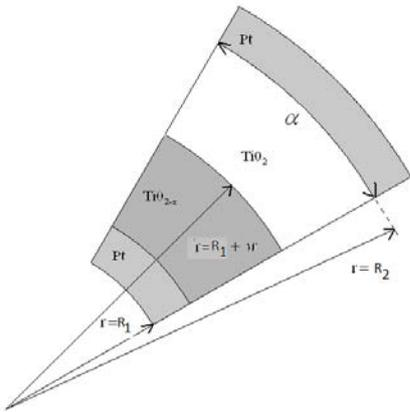
Figure 3. The cylindrical-cut memristor topology during doping
