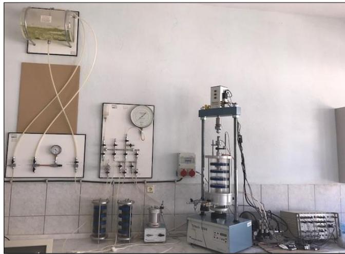
Figure 5. Dynamic triaxial test system
