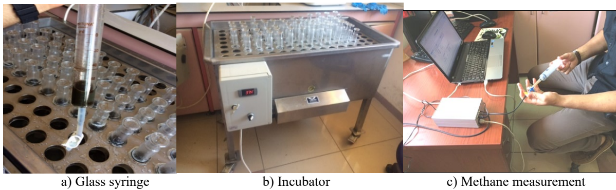
Figure 3. Glass syringe, incubator and methane measurement
