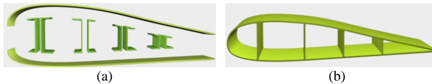
Figure 12. a) traditional production of composite parts, b) net shape, single part composite production (URL 4)
