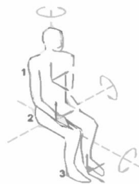
Figure 1. Position of Accelerometer According to ISO Standard (Point 2)
