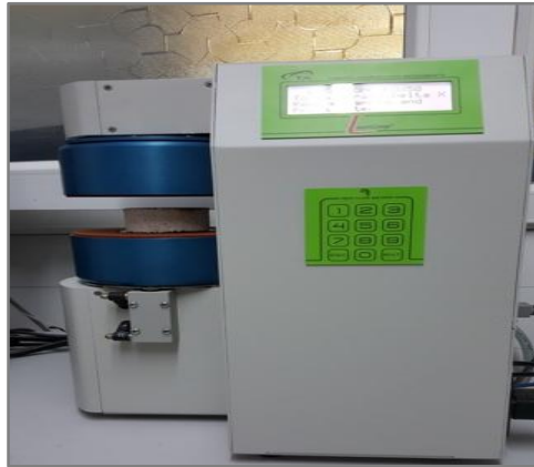
Figure 4. Thermal Conductivity Coefficient ( \lambda ) Measurement
