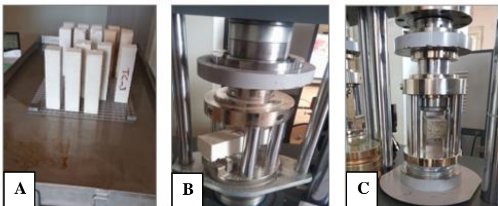
Figure 3. Performing The Experiments A: Capillary Water Absorption, B: Flexural Strength, C: Compressive Strength
